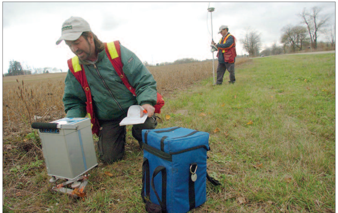
Gilles Bergeron and Luc Houle use a device that measures tiny changes in gravity caused by changes in the distance from the surface to bedrock.
